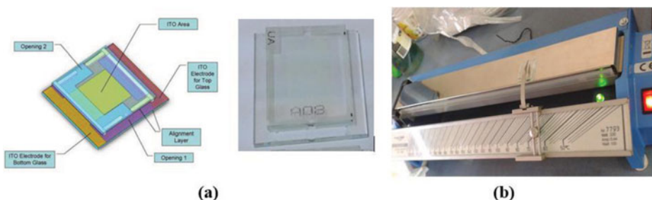
Figure 4. (a) The structure and photography of empty LC cell (b) Filling LC cell with capillary effect.
